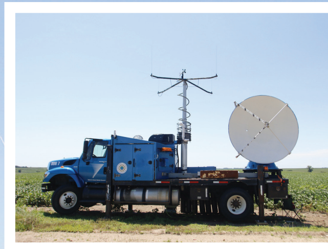
One of three Doppler on Wheels radar trucks used for the GRAINEX research project.
