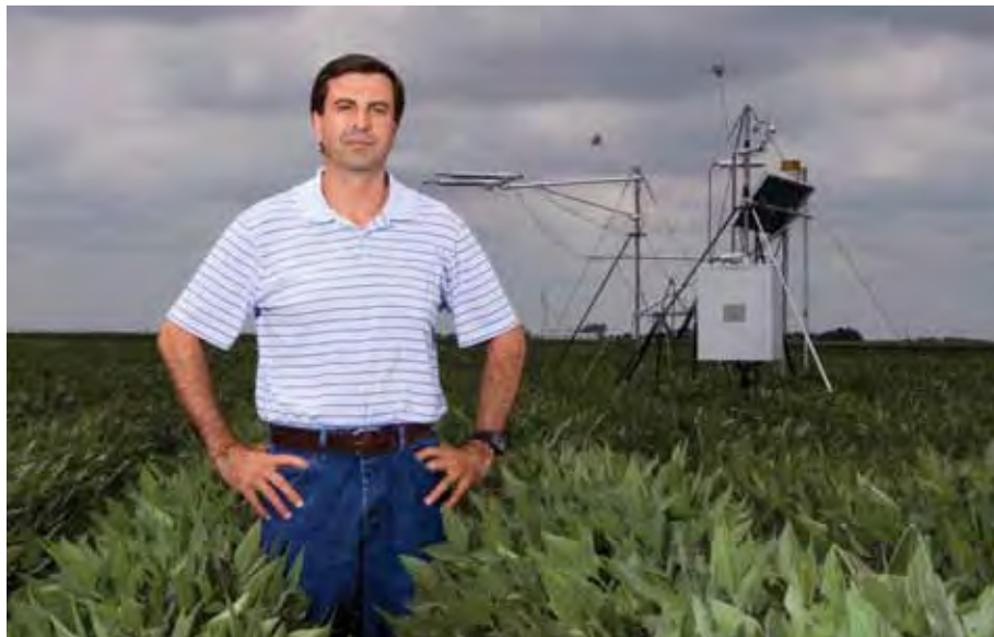
Suat Irmak checks sensing equipment in a soybean field near Geneva. By measuring the moisture leaving a field of crops, Irmak provides farmers with information that can help conserve energy and water, save money and ultimately grow better crops.
